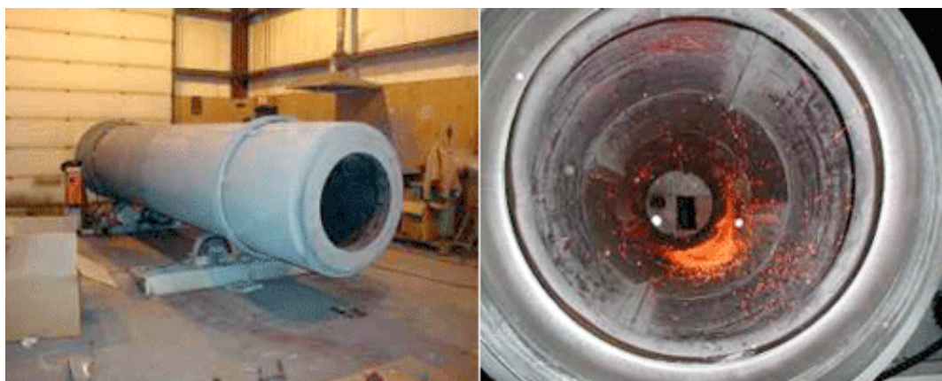
Picture 4 - The Rotary Kiln - External and Inside Views (left and right)
